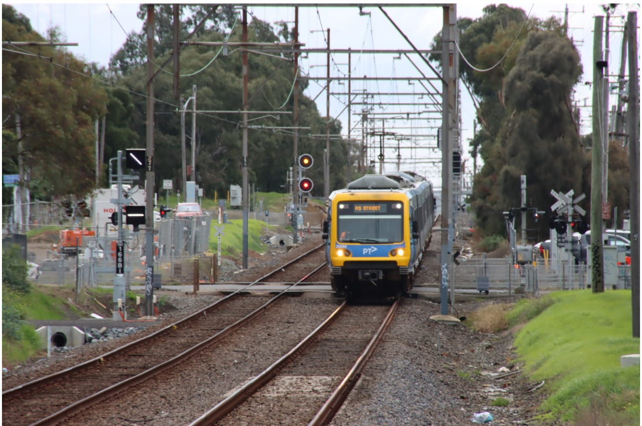
More photos from the resignalling associated with the provision of the single line viaduct between through Bell and Preston. (Above left) The Down outer Home signal protecting the single line, TBY166, is situated well south of Thornbury. Although the Home is situated in roughly the same location as a previous Automatic, the sighting of the Home is badly obstructed by the overhead structures. A banner indicator, TBY166BI, is consequently provided on dead straight piece of track. (Below) Another view of Home TBY166/Banner Repeater TBY166BI with the road set through the single track section, but the with entry Home into the section at stop. If the Signaller had only set the route into Thornbury platform, but not into the single track section, Home TBY166 would show Medium Speed Warning. (Above right) The new style of signal post telephones that are appearing around the Metropolitan area. (Photos: Andrew Waugh)
