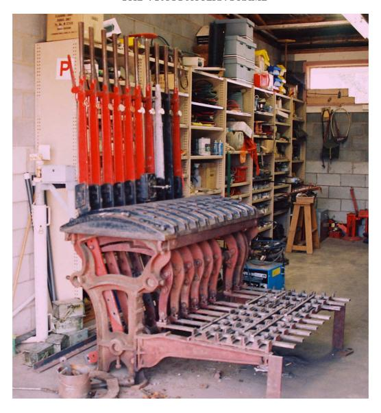
These photos were taken by David Langley and show the 1995 'A' pattern frame for Wallan in the course of erection in the Signal Depot at Seymour and give an excellent idea of the design of the frame.
