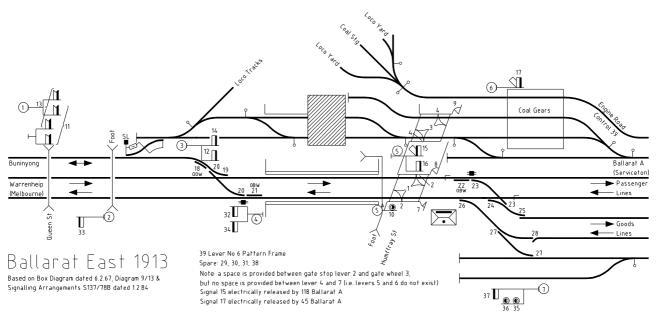
A box. The two arms on the left hand doll on Post 7 had been replaced by discs, and the dead end staff locked siding off the Buninyong line at the rear of the Engine Shed had been removed.
