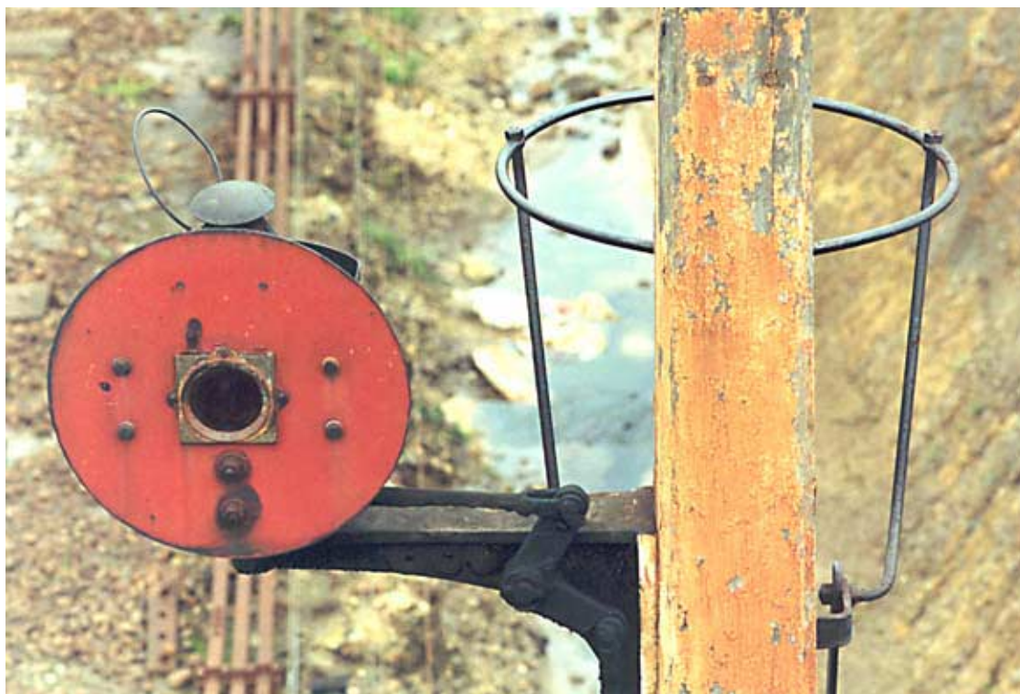
The wall bracket disc at Danger. Disc 13 (Post 33) at Ballarat B box controlled set back moves from the Down line to the four main lines through the train shed. The post and disc was provided on 22 December 1910; and when these photos were taken nearly 80 years later it is unlikely that either had been altered significantly since. The large red disc gives a clear 'on' signal during the day with a small glass in the centre of the disc giving a red light at night.
