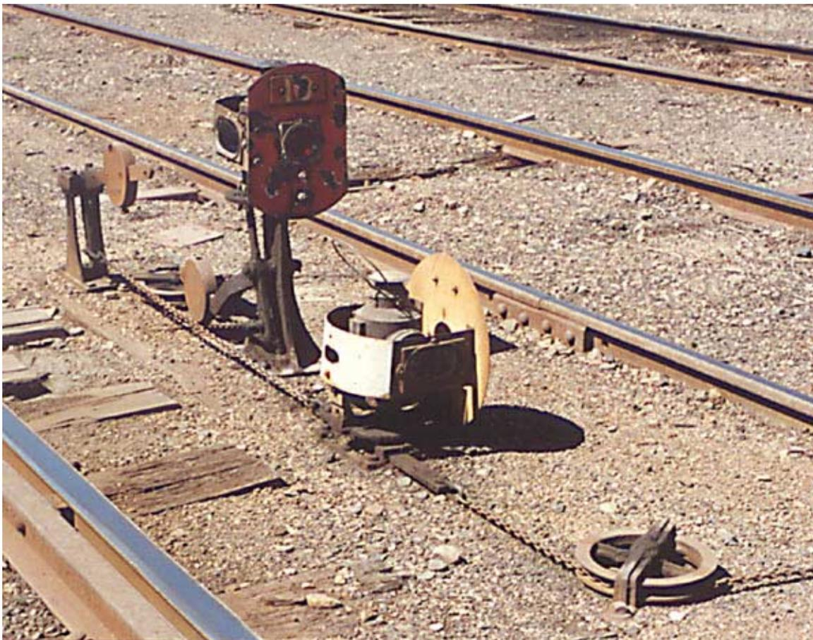
where it was required to signal two separate routes past a location. Such signals were described in the quaintly formal language of the 'Book of Signals' as 'Two Ground Disc Signals, one above the other'.
