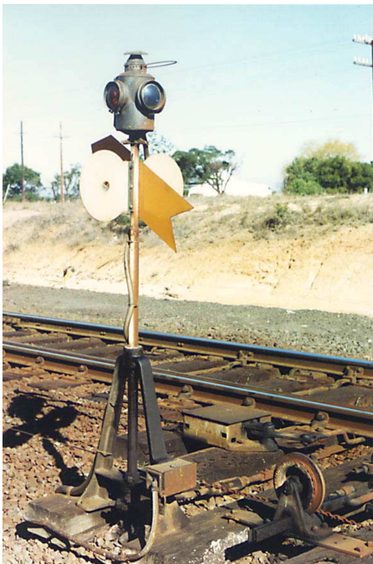
(Above) The diagram of the Victorian Double Wire switchstands published in WN 42/29 (Below) The switchstand on the Down end points at Lethbridge in May 1988. The photo is taken from the front quarter and both the two white discs and the yellow arrow can be seen. When this photo was taken the switchstands at Meredith, Lethbridge, and Lal Lal were still equipped with lamps however the conduit snaking up the staff indicates that an electric lamp has been provided.
