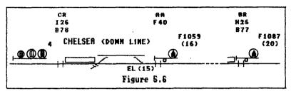
15 seconds. An unusual feature here is that as the stopping outer approach for the boom barriers at Bondi Road, Bonbeach (BR), commences immediately on the Down side of the Argyle Avenue crossing, the next signal along, F1087 (Bonbeach 4), must also be controlled by Chelsea to prevent a shunting movement from unnecessarily holding down the booms behind an Up train.
