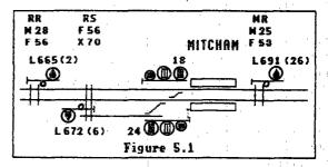
the signal lever is put back while a train is in the approach section; this provision allows for the possibility that in these circumstances the train might not be able to stop before reaching the crossing.
