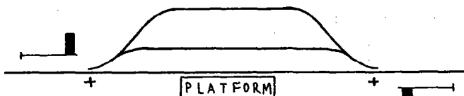
Fig. 1. Plunger locked crossing loop.
