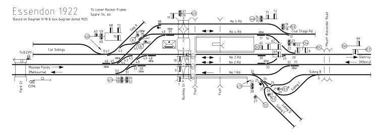
of these were through trains. Presumably, No 1 Road was used for Up trains originating from Broadmeadows, No 3 Road for Down through trains to Broadmeadows, and No 4 Road for terminating trains. Three trains stabled over night at Essendon – two would have stabled in the Car Sidings, and the third (the last Up service from Broadmeadows) probably stabled in the Back Platform or in No 5 Road.
