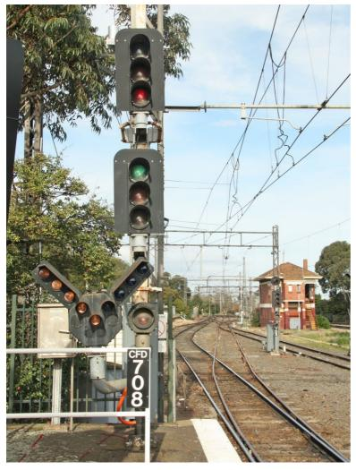
(Left) As noted in the signalling alterations sections, the two feather route indicators at Caulfield were replaced by theatre route indicators on 23 August 2015. This photo of one of the indicators, on Home CFD708, was taken on its last day of service. CFD708 is on Platform 4 and is normally used only for Down Dandenong services, and so the right hand feather is rarely used.
